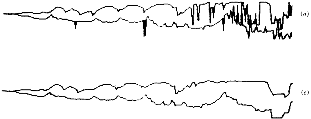
FIGURE 2. Stages in preprocessing one frame (for (a-c) see plate 1): ( a ) digitized image; ( b ) filtering; ( c ) thresholding; ( d ) edge detection; ( e ) edge smoothing.
